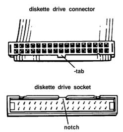
Align the connector with the socket so the tab on the connector lines up with the notch in the socket. Make sure the holes in the connector fit over all the pins in the socket and then push in the connector.
